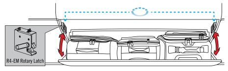
Compared to mechanical latching solutions or solenoid-driven mechanisms traditionally used in these applications, Southco's electronic access solutions (EAS) not only offer proven reliability, they also offer space and power reduction capabilities that can help to reduce the overall operational footprint of an aircraft. Gear motor-operated electronic locks, such as
